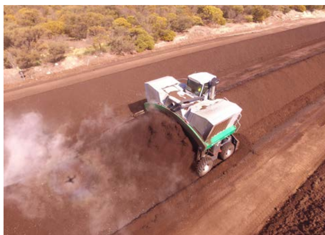
Figure 2 Windrow turner. Image: Peats Soil & Garden Supplies.
